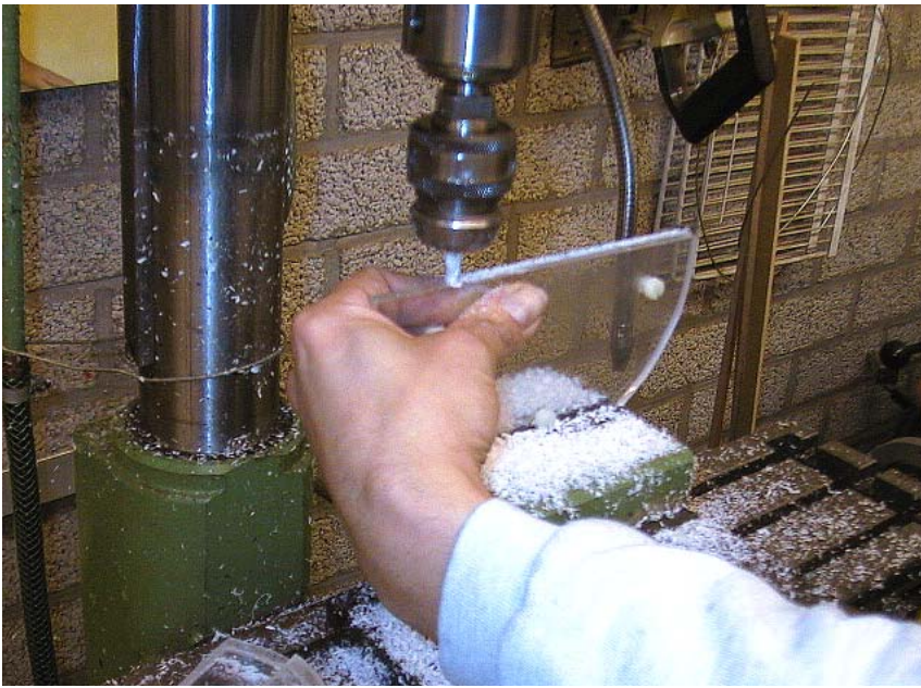
Figure 7. Milling the grooves in the Perspex semicircles.
